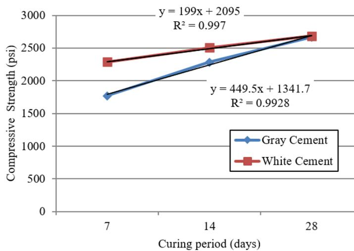
Fig. 6. Compressive Strength of concrete made with gray and white cement [W/C: 0.45 Mix ratio: 1:1.5:3]
