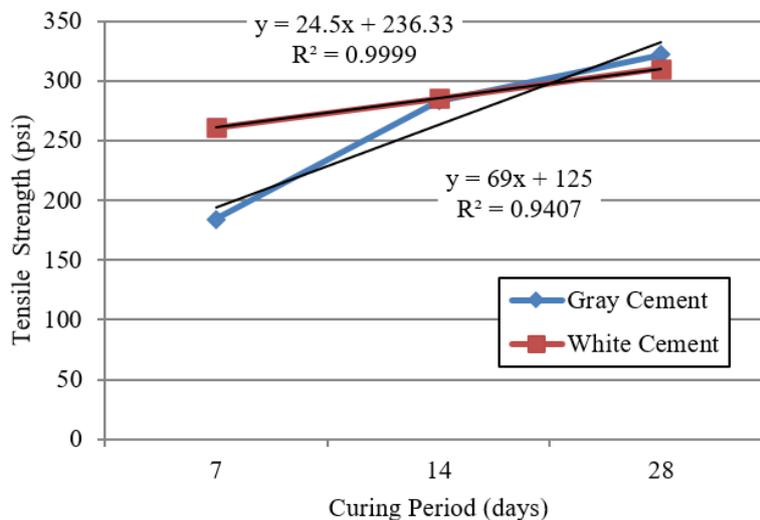
Fig. 10. Tensile Strength of concrete made with gray and white cement [W/C: 0.45 Mix ratio: 1:1.5:3]
