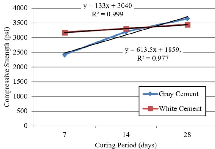
Fig. 3. Compressive strength comparison of concrete made with gray and white cement. [W/C: 0.40 and Mix ratio: 1:1.25:2.5].
