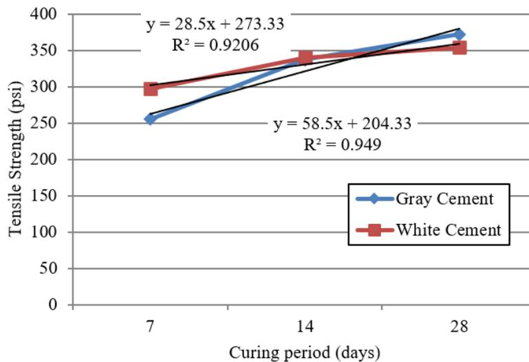
Fig. 8. Tensile Strength of concrete made with gray and white cement [W/C: 0.45 Mix ratio: 1:1.25:2.5]
