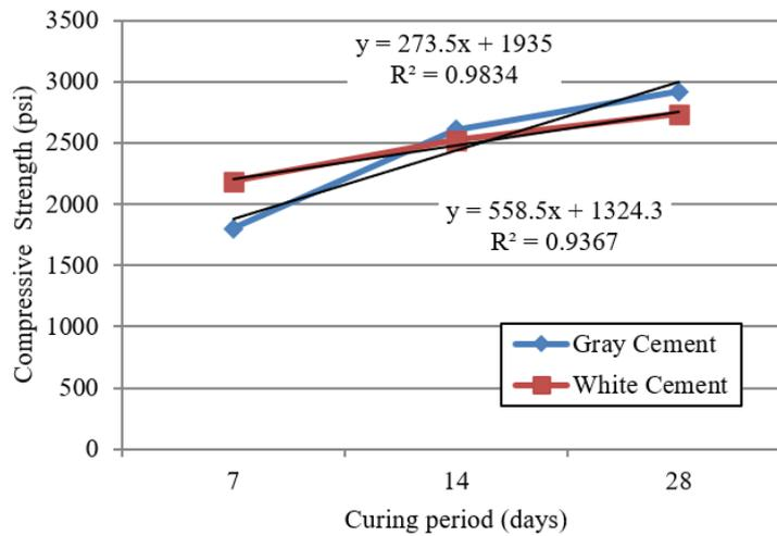
Fig. 5. Compressive Strength of concrete made with gray and white cement. [W/C : 0.40 Mix ratio: 1:1.5:3]
