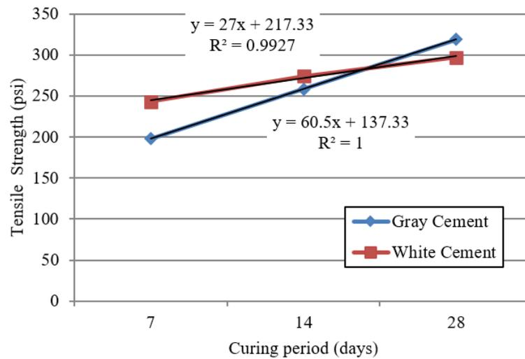
Fig. 9. Tensile Strength of concrete made with gray and white cement [W/C: 0.40 Mix ratio: 1:1.5:3]
