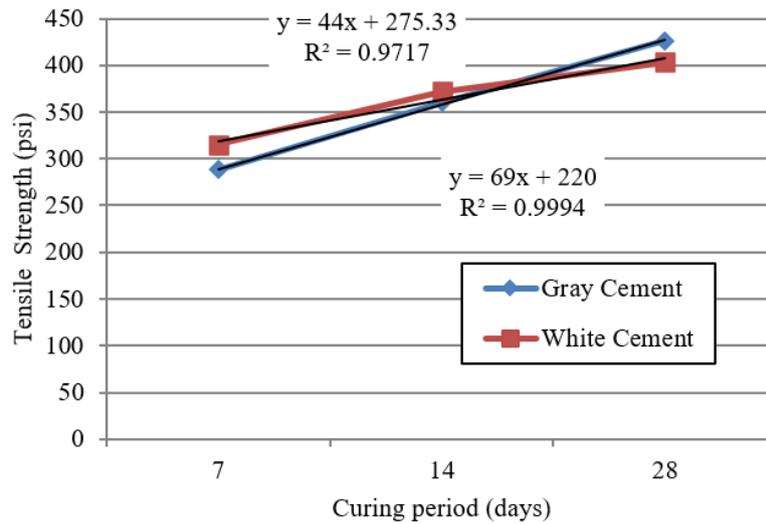
Fig. 7. Tensile Strength of concrete made with gray and white cement [W/C: 0.40 Mix ratio: 1:1.25:2.5]
