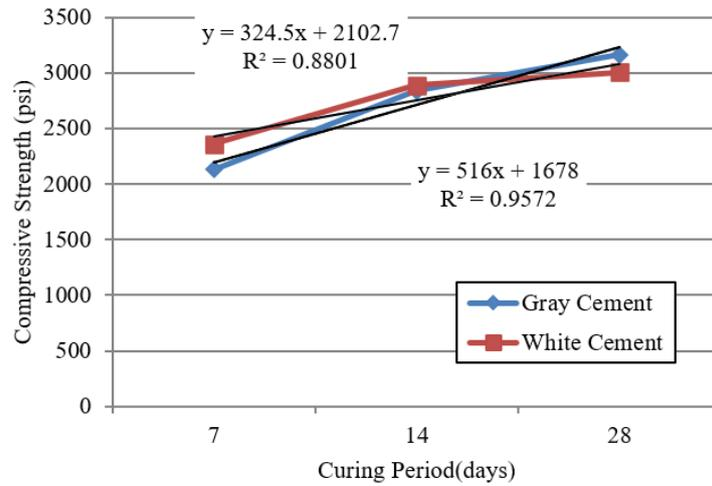
Fig. 4. Compressive strength of concrete made with gray and white cement [W/C: 0.45 Mix ratio: 1:1.25:2.5]
