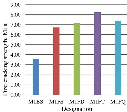
Fig. 2. Effect of multiple layers of wire mesh on the cracking strength
