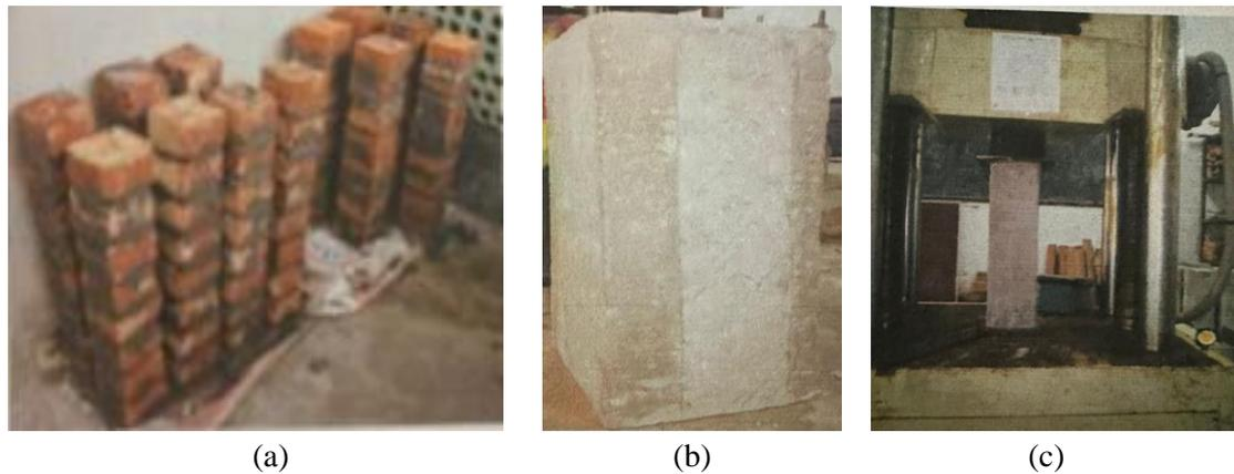
Fig. 1. (a) Brick masonry column (b) strengthened brick masonry column and (c) experimental setup.
