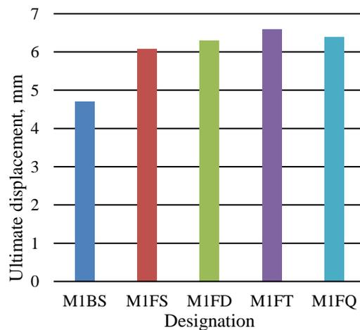
Fig. 3. Effect of multiple layers of wire mesh on the displacement.
