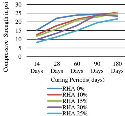
Fig. 3.3. Compressive strength of different RHA concretes in NaCl environment.
