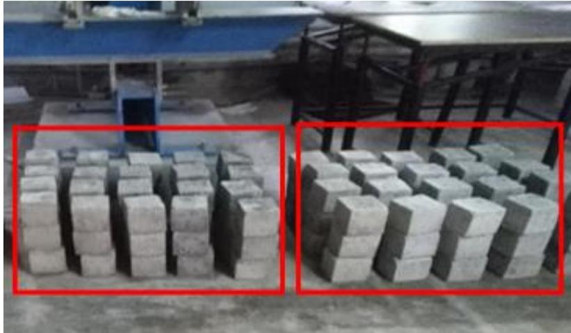
Fig. 3.1. From left, specimens exposed to sodium chloride environment and specimens exposed to plain water.
