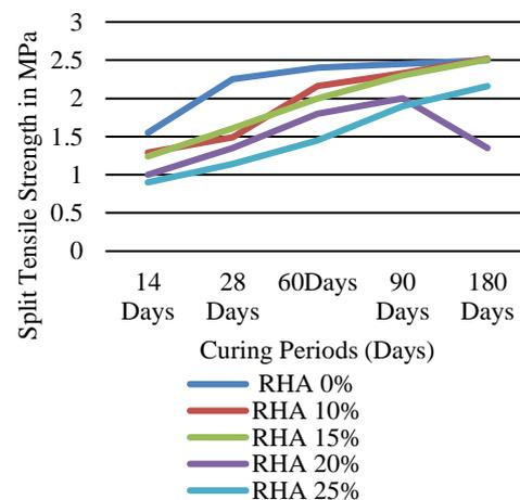
Fig. 3.5. Split tensile strength of different RHA concretes in NaCl environment.
