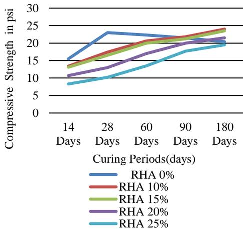
Fig. 3.2. Compressive strength of different RHA concretes in PW environment.
