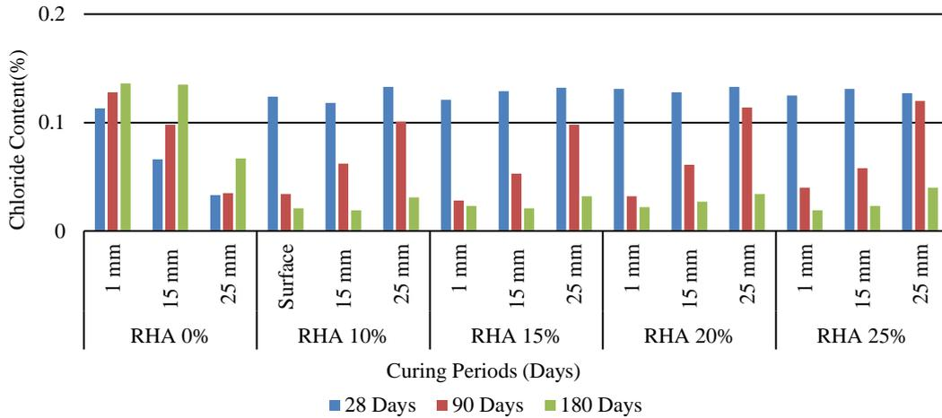
Fig. 3.6. Chloride content (%) at different depth levels of RHA concretes in NaCl environment.
