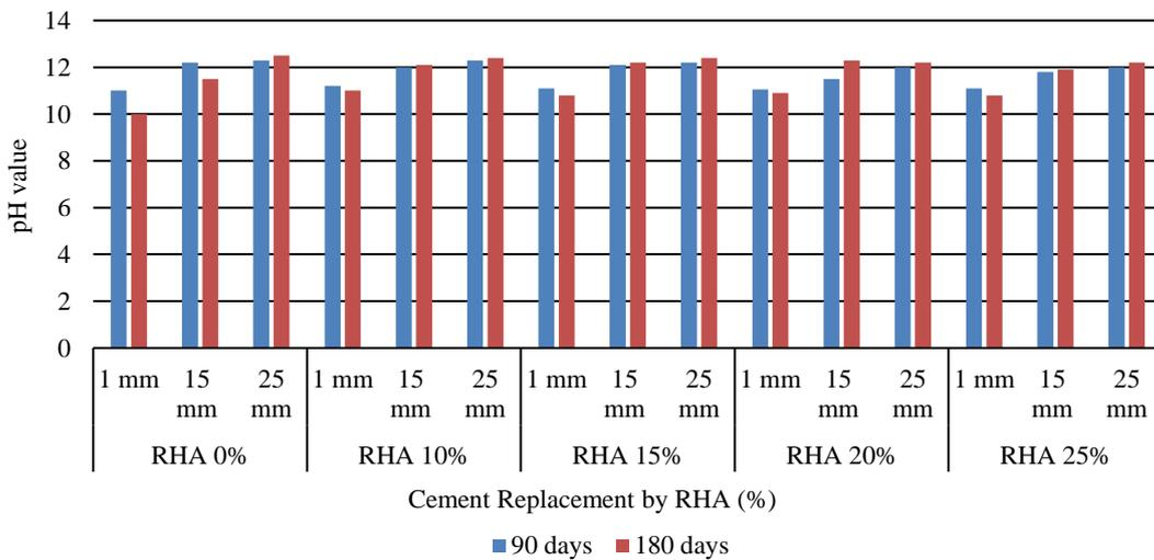
Fig. 3.7.  $p^H$  values of RHA concretes at different depth levels in NaCl environment.
