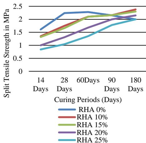
Fig. 3.4. Split tensile strength of different RHA concretes in plain water.
