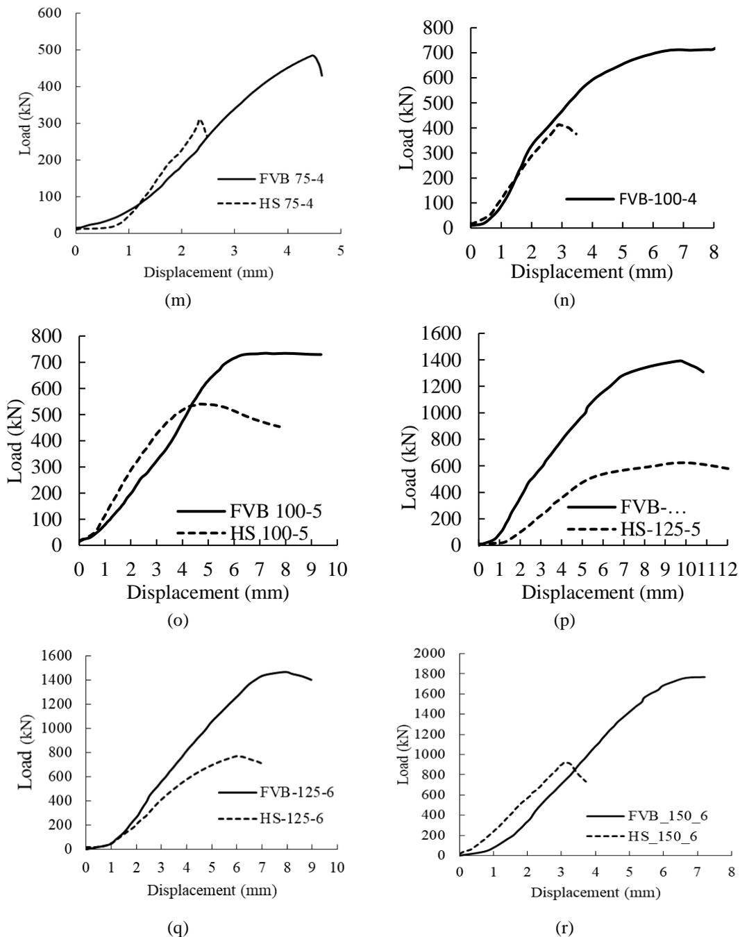
Fig. 8. Load displacement relation of hollow and filled specimen.
