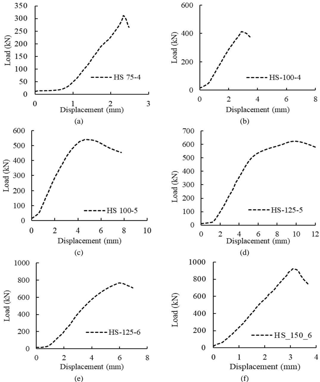
Fig. 6. Load displacement relation of hollow specimen.
