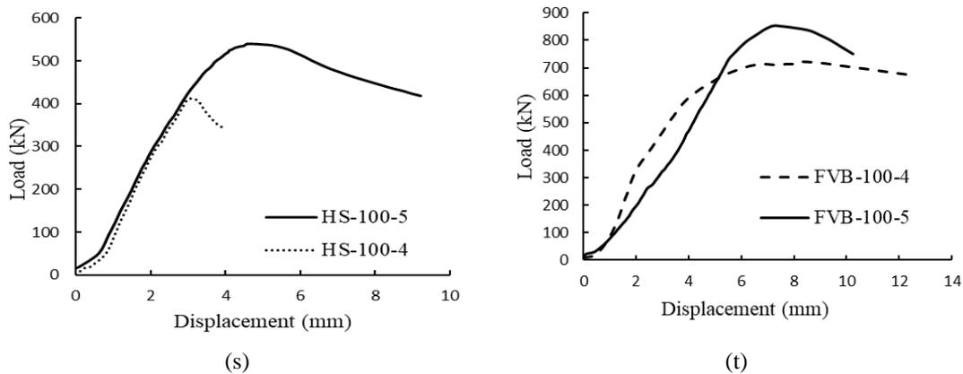
Fig. 9. Load displacement relation of 4mm and 5mm plate hollow and filled specimen.
