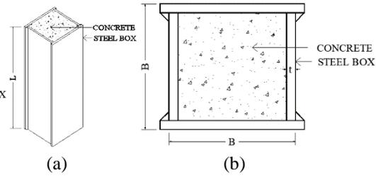
Fig. 3. Filled specimen (a) cross section (b) isometric view
