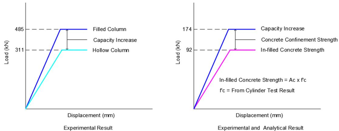
Fig. 1. Schematic Graph illustrate the concrete confinement strength of specimen -1.
