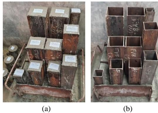
Fig. 4. a) Hollow specimen b) Filled specimen
