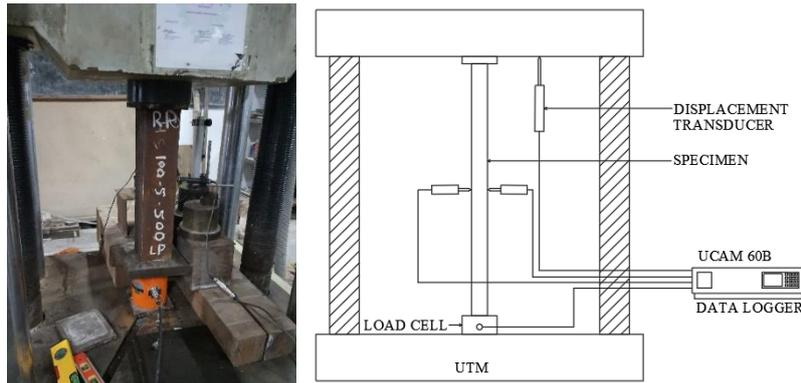
Fig. 5. Instrument setup.
