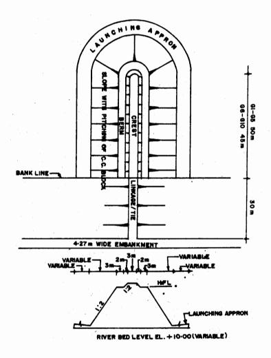
Fig 2. Plan and Section of the Spur
